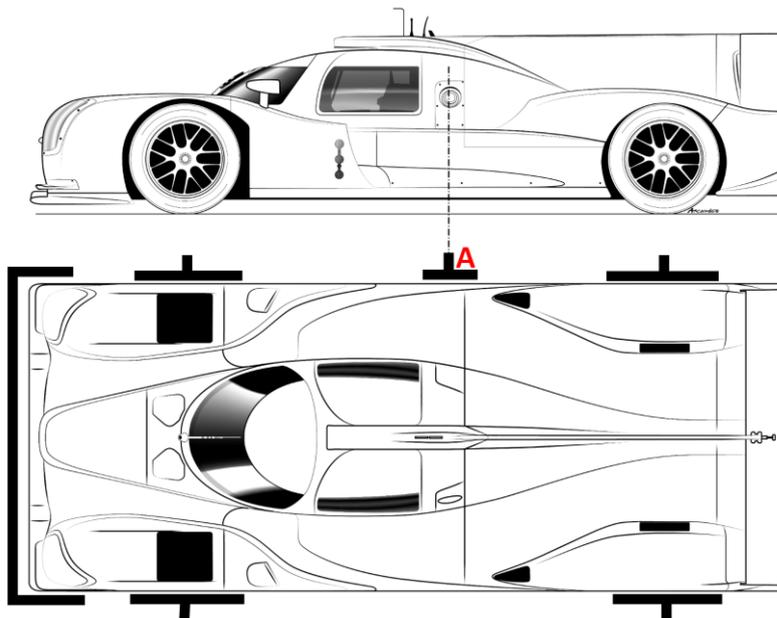
For practical reasons, the competitors shall prove FIA/ACO the difference in altitude between the described point 'A' above and the altitude of the ground at the vertical of the foremost (closest to fast-lane) point of the fuel rig (in the vertical plane, perpendicular to the pit lane line and passing through the centre of the tank).
